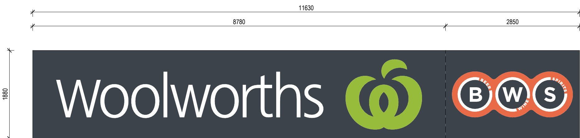
S 2.2b EXTERNAL FACADE SIGN COMBINED SIGN 11630mm x 1880mm OVERALL. (1500mm HIGH WW LOGO). INTERNALLY ILLUMINATED SIGN. MOUNTED TO FACADE OF BUILDING.
