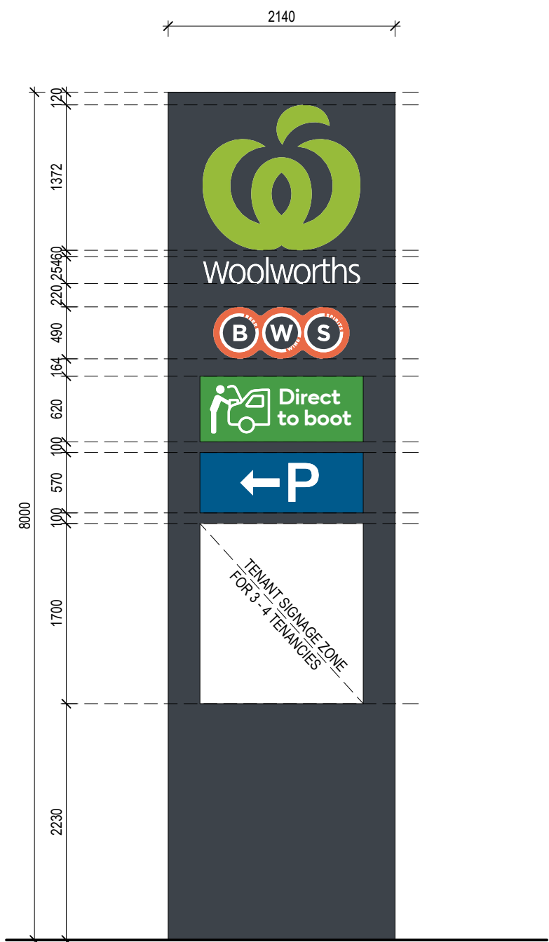
S 1.1 WOOLWORTHS PYLON SIGN - 8m SPECIAL SIGN 8000mm x 2140mm x nom. 600mm. DOUBLE SIDED. INTERNALLY ILLUMINATED SIGNAGE ELEMENTS. MOUNTED TO GROUND.
