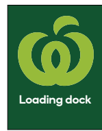
S 1.7 CARPARK SIGNAGE - LOADING DOCK PANEL SIGN 930mm x 1200mm. MOUNTED ON WALL. SINGLE SIDED.
