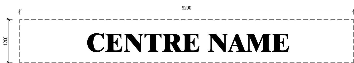
S 2.5 CENTRE BRANDED SIGN 'AUSTRAL NORTH VILLAGE' BACK-LIT METAL SIGNAGE. MOUNTED TO FACADE. INTERNALLY ILLUMINATED SIGNAGE ELEMENTS.
