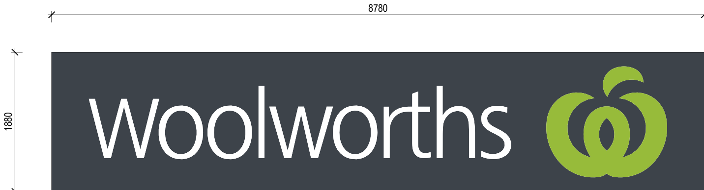
S 2.2a EXTERNAL FACADE SIGN FACADE SIGN 8780mm x 1880mm OVERALL. (1500mm HIGH WW LOGO). INTERNALLY ILLUMINATED SIGN. MOUNTED TO FACADE OF BUILDING.
